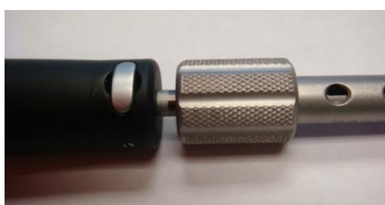
Figure 5 The top of the knob on the outer shaft is resting just below the laser mark line on the inner shaft.
